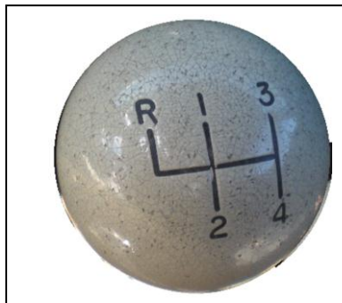
Original Hurst shifter ball – White the distance between the 1 and R is greater then on the after market one.
