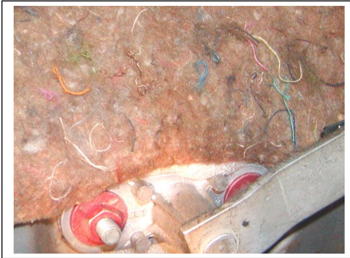
Original under dash cowl insulation. It is beige in color with large multi color thread fibers
